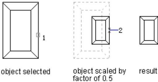
You can also scale objects by comparing the basic scale and new scale. The objects become larger if the new scale is large than the basic scale. The dimension will be scale along with the object to scale.
