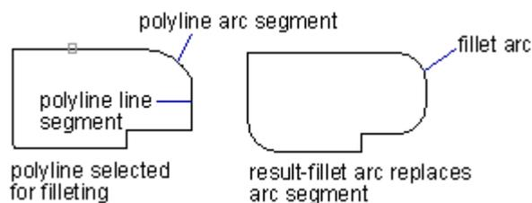
When the fillet radius is set to 0, no fillet arcs are inserted. If two polyline segments are separated by one arc segments, system deletes this arc segment and extends the lines to intersect with each other.
