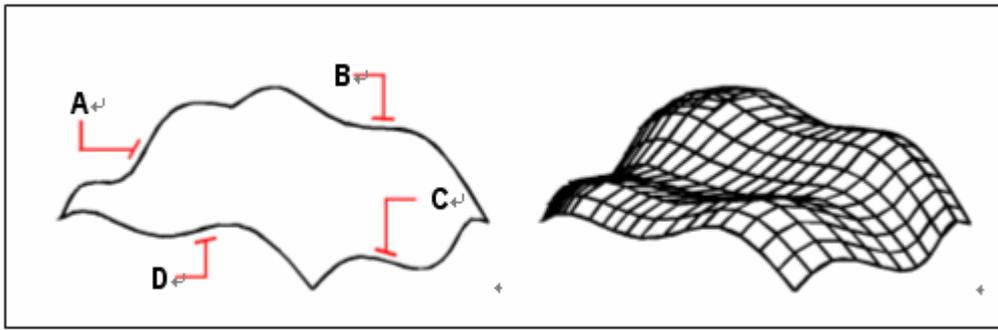
Select the objects to be used as the four edges (A, B, C, and D). The resulting Coons surface patch mesh.
