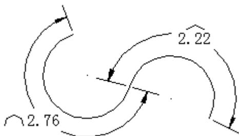
Additionally, orthogonal or radial extension line is available for arc length dimension, only the included angle of the arc segment selected for creating arc length dimension is smaller than 90 degree can display it's orthogonal extension line.
