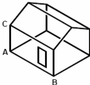
Define the new UCS by selecting the origin (**A**), a point on the positive x-axis (**B**), and a point in the positive y direction (**C**).
