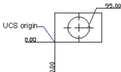
In ordinate dimensions, the dimension text is always aligned with the ordinate leader line, ignoring the text orientation defined by the current dimension style. You can also supply your own text or accept the default one.
