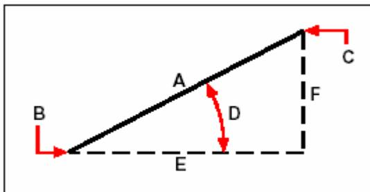
Use the Distance command to calculate the distance (**A**) between two points (**B** and **C**), the angle in the xy plane (**D**), the angle from the xy plane, and the delta x (**E**), delta y (**F**), and delta z distances between the two points.
