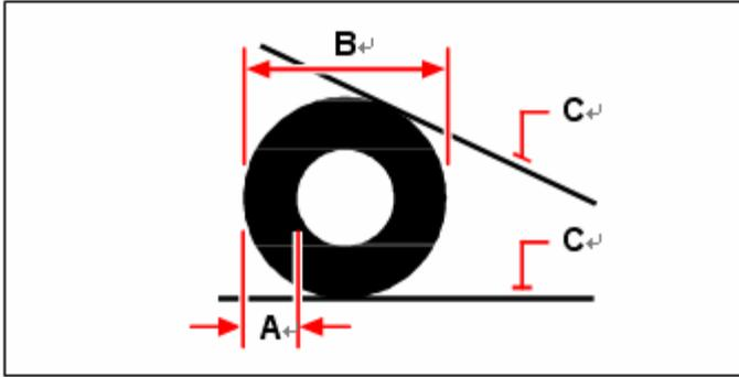
Width (**A**) and diameter (**B**) of the donut and tangent objects (**C**).
