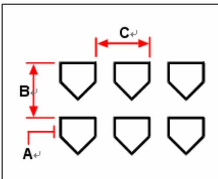
To create a rectangular array, select the object to copy (**A**), type the number of rows and columns, and then specify the distance between each row (**B**) and column (**C**).
