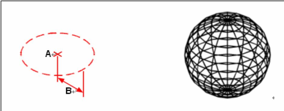
Center (**A**) and radius (**B**) of the sphere.      The resulting sphere.
