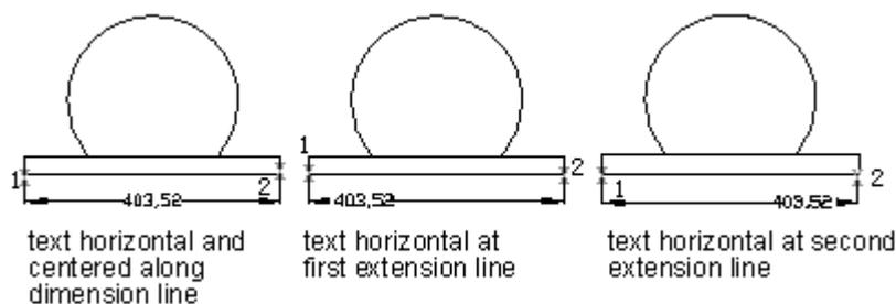
If the “place text manually when dimensioning” option on the Fit tab of the Modify Dimension Style dialog box is chosen, as you create dimensions, you can place the dimension anywhere inside or outside the extension lines along the dimension line. This option is useful when the space between the extension lines is limited.
