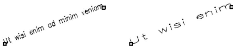
Text aligned between two points    Text fit between two points expands or maintains a constant height/width ratio    compresses to fit
