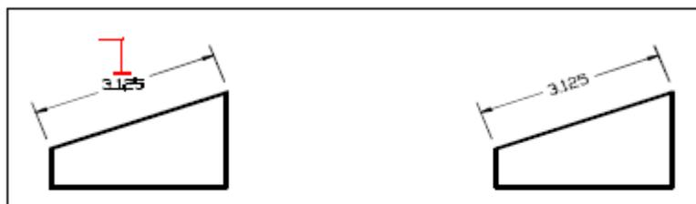
Select the dimension to be rotated (A), and then type the rotation angle.
