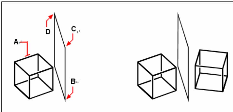
Select the object to mirror (**A**), and then specify the first point (**B**), second point (**C**), and third point (**D**) defining the mirror plane.
