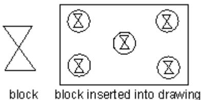
**To insert an entire drawing into the current drawing**
