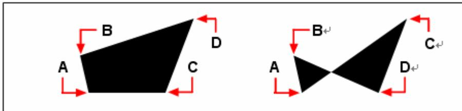
After you select the first two points (**A**) and (**B**), the sequence in which you select the third (**C**) and fourth (**D**) points determines the shape of the resulting quadrilateral plane.
