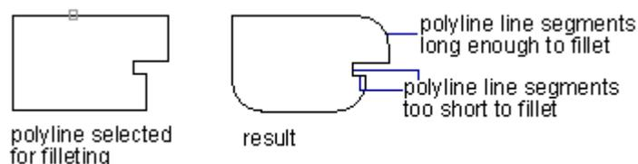
The fillet arcs replace arc segments when the fillet radius is greater than the radius of the arc. As shown in the illustration:
