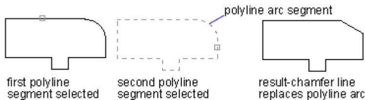
**To chamfer selected vertices in a polyline**
