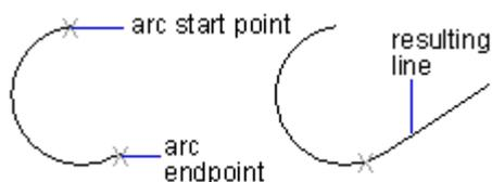
You can connect sequentially drawn arcs in the same way. To create connected arcs using a menu, click Arc from the Draw menu, and then click Continue. In both cases, the resulting object is tangent to the previous one. You can use the shortcut menu to repeat the Continue option.
