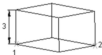
RECTANG or PLINE command creates a rectangle or closed polyline from which you can create a box using EXTRUDE. The 3D command creates a box shape defined by surfaces only.
