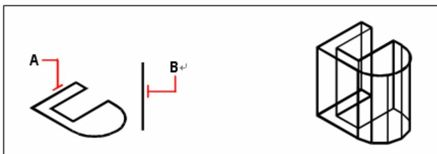
Select the object to extrude (**A**) and the extrusion path (**B**). The resulting extruded surface mesh.
