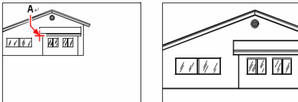
Current view(left) showing the point to be centered in the new view (A), and the new view(right) zoomed using a scale factor of 2x
