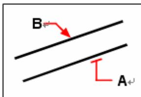
To make a parallel copy passing through a point, select the object to copy (**A**) and then specify the through point (**B**).
