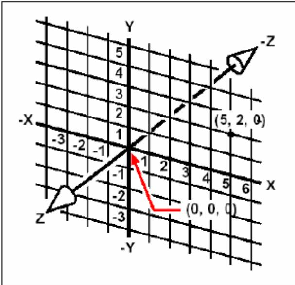
Each position in the CAD drawing has its corresponding x,y,z coordinates within Cartesian Coordinate System. Point 5,2,0 is 5 units to the right (along the x axis), 2 units up (along the y axis), and 0 units (along the z axis) from the origin (the 0,0,0 point). Settings such as snap and entity snap allow you to draw accurately without specifying coordinates.
