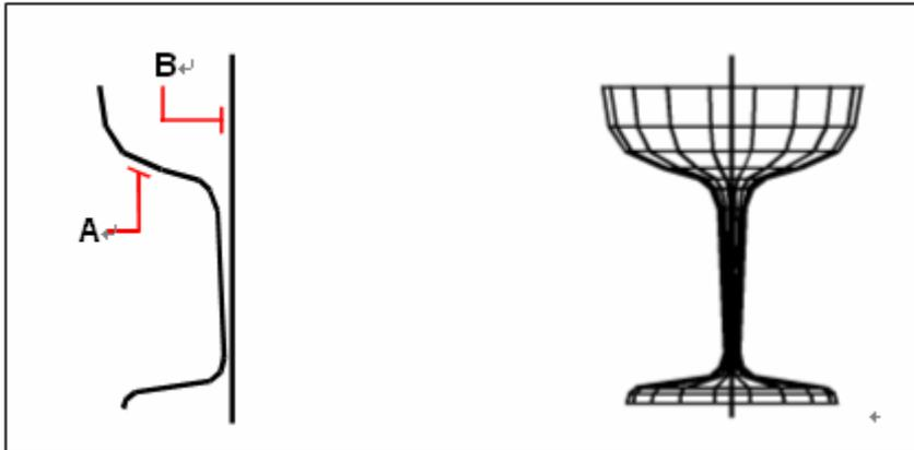
Select the object to be revolved (**A**) and the axis of revolution (**B**). The resulting revolved surface mesh.
