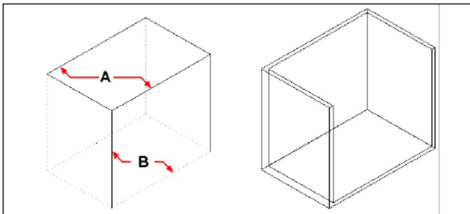
Select the entity, and then select faces to remove (A) and (B), then specify an offset distance.
