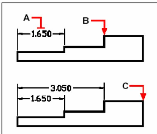
To add a baseline dimension to an existing linear dimension, select the existing dimension (A), select the next extension line origin (B), and select as many additional points as you want (C).
