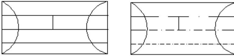
For polylines, you can use system variable `PLINEGEN` to control whether a linetype pattern is centered on each segment or is continuous across vertices throughout the entire length of the polyline.
