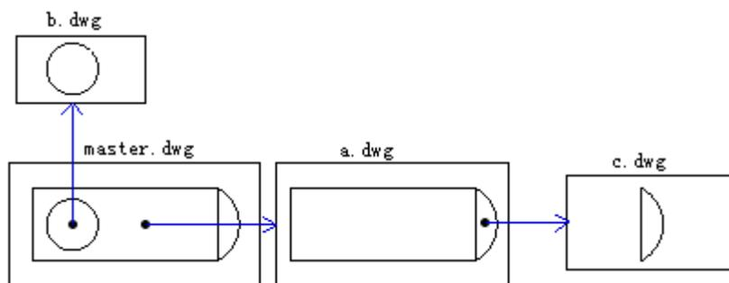
Specify the type of xref, including attach and overlay. Using overlay to exclude any nested xrefs rather than overlay xrefs. This type is typically used for sharing data in network. In Xrefs that are attached in overlay type, you can viewed relative methods directly between the drawing and other grouping drawings.
