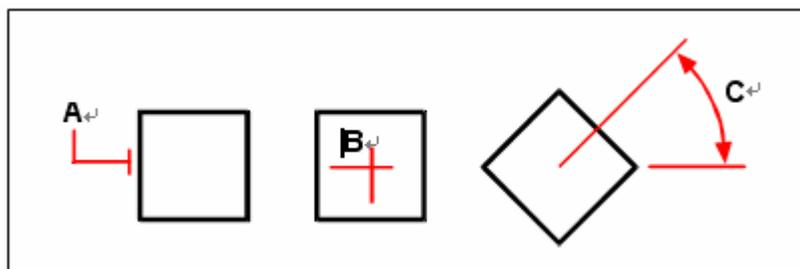
To rotate an object, select the object to rotate (A), and then specify base point (B) and the rotation angle (C).
