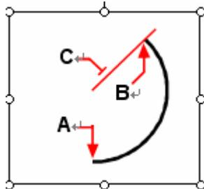
Start point (A), endpoint (B), and included angle (C).
