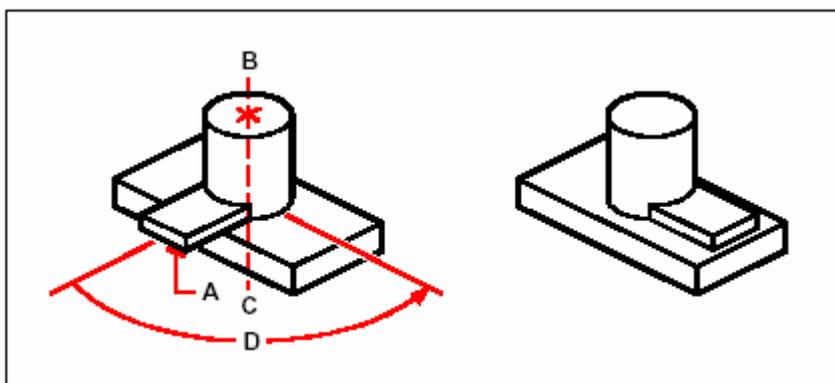
Select the objects to rotate (**A**), specify the endpoints of the axis of rotation (**B** and **C**), and then Result after rotating the objects
