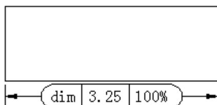
In which, inspection tag, used for mark the text of dimension inspection is located at the left side within the inspection frame.
