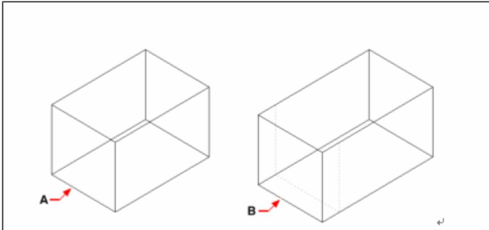
Select the entity to extrude, and then specify the face(s) to extrude (A), and the height of extrusion or path. The resulting entity with the face extruded to position (B).
