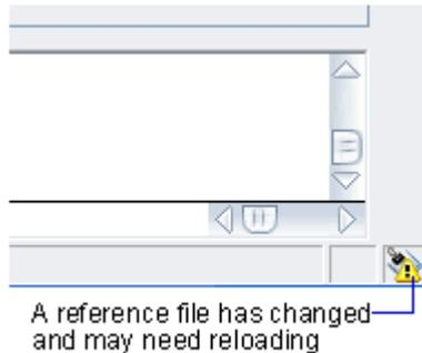
By default, modified xrefs will be checked every five minutes. You can change the time intervals by setting the XNOTIFYTIME system registry variable using (setenv "XNOTIFYTIME" "n") where n is a number of minutes between 1 and 10080 (seven days). Note that XNOTIFYTIME value must be entered by ignorecase.
