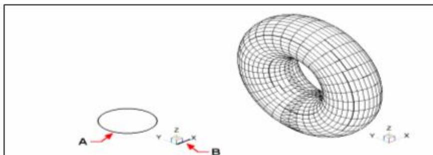
Select the object to revolve (**A**) and the axis (**B**) about which to revolve it. followed by the angle of revolution. The resulting revolved solid.
