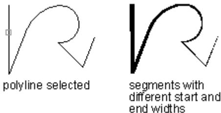
You can change the width of an entire polyline, applying a uniform width to the polyline or assigning tapering width with gradient size.
