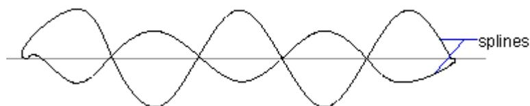
Multiple points are required for drawing irregular splines. And you can close the spline so that the start and endpoints are coincident and tangent.
