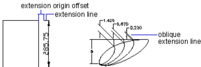
The first extension line lies on the side where you specified the first extension line origin. If you create a dimension for a line, you do not specify the extension line origin. Because the endpoint of the line closet to the specified point becomes the origin of the first extension line. Generally, the extension lines are perpendicular to the dimension line. However, if there is not space, you can make them oblique, shown as the figure above.
