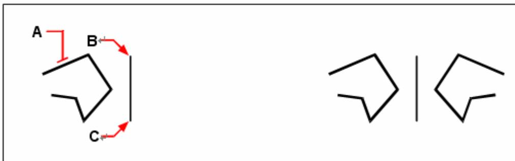
To mirror an object, select it (A), and then specify the first point (B) and second point (C) of the mirror line. Result.
