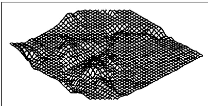
An example of a three dimensional terrain model created using rectangular meshes. The following picture shows the polygon mesh with coordinates specified for each vertex.
