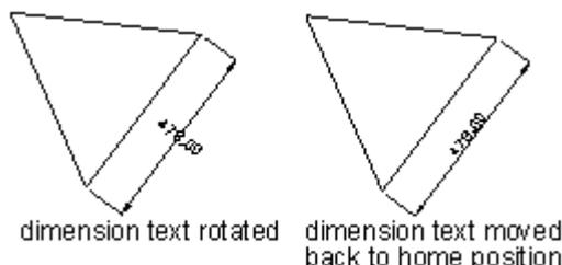
You can rotate the specified text at an angle using the Dimension-Align Text-Angle option, or change the angle and content in the Properties panel.
