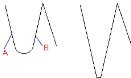
Select the polyline along the (A) and (B) segments. Result after chamfering.
