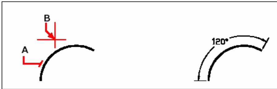
To dimension the angle subtended by an arc, Select the arc (A), and then specify the dimension arc location (B).
