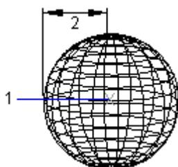
To create a dome or dish, combine a sphere with a box and use SUBTRACT. If you want to create a spherical object with additional details, create a 2D profile and use REVOLVE to define a rotation angle about the Z axis. 3D command creates a spherical shape defined by surfaces only.
