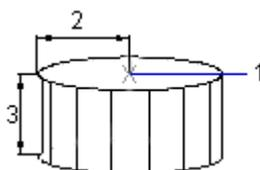
You can draw a circle and then use EXTRUDE to create a solid cylinder. To construct a cylinder with special detail, such as grooves along its sides, you can create a 2D profile of its base with a closed PLINE and then use EXTRUDE to define its height along the Z axis.
