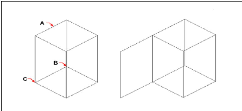
Specify the face(s) to copy (**A**), the base point (**B**), and the end point(**C**). The resulting entity with the face copied.
