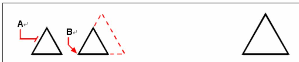
To scale an object by a scale factor, select the object (**A**), and then specify the base point (**B**) and the scale factor.
