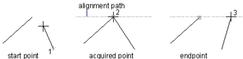
By default, the object snap tracking is set to Orthogonal. Alignment paths and tooltips are displayed at 0, 90, 180, and 270 degrees from acquired object points. However, you can use polar tracking angles instead on the Polar Tracking tab in the Draft Settings dialog box.
