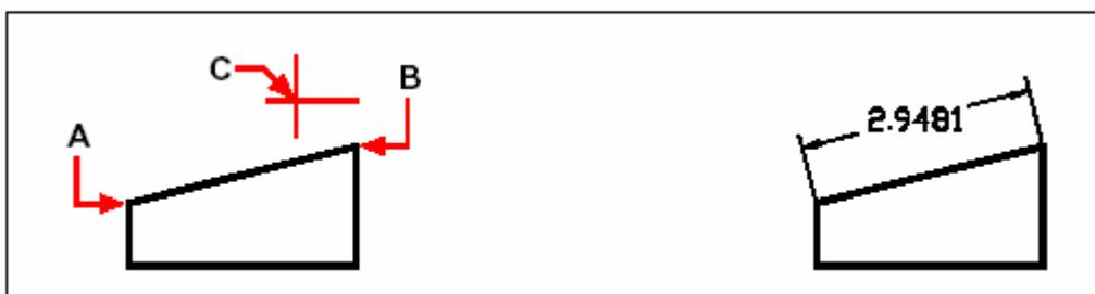
To insert an aligned dimension by selecting the extension line origins, select the first extension origin (**A**), select the second extension origin (**B**), and then specify the dimension line location (**C**).
