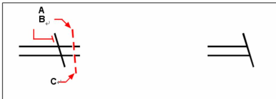
Select the boundary edge (**A**), and then specify the first point (**B**) and second point (**C**) of the fence. Result.
