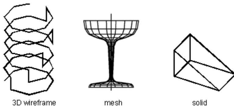
You should notice that different editing manipulations result in different visual effects because of various model and creating methods. You should avoid mixing the models of different type when creating 3D objects. Limits are also applied to the conversion of model types, only solid-curve and curve--wireframe conversion are available.
