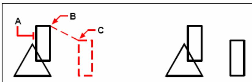
Object to copy (**A**), base point (**B**), and displacement point (**C**). Result.
