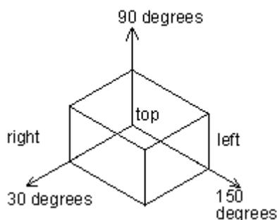
In addition to using ISOPLANE command to switch isometric planes, you can also use shortcut key F5 or CTRL+E. specifying one of the three isometric planes results in Ortho and crosshairs to be aligned along the corresponding isometric axes.
