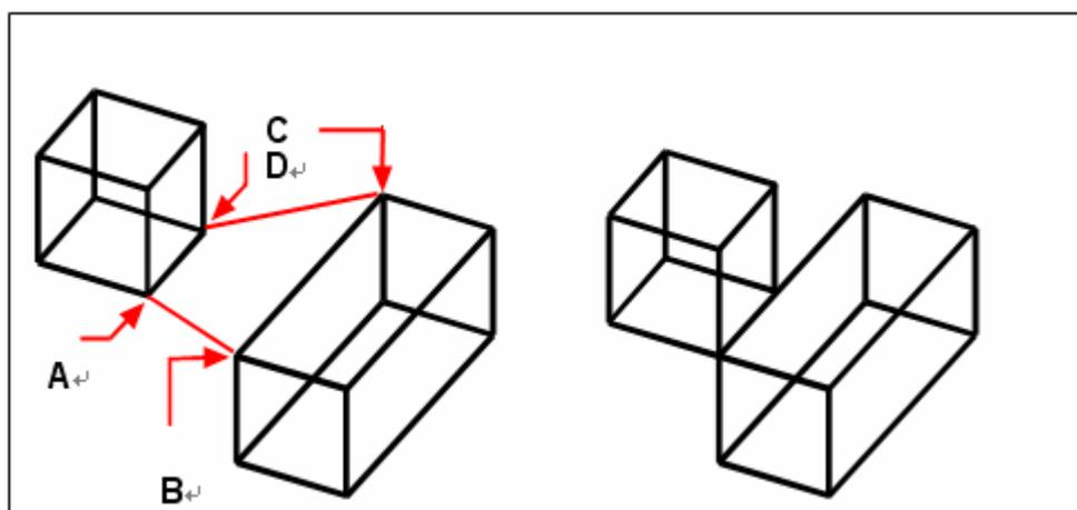
Select the objects to align, and then specify the first source point (**A**), the first destination point (**B**), the second destination point (**C**), and the second destination point (**D**).
