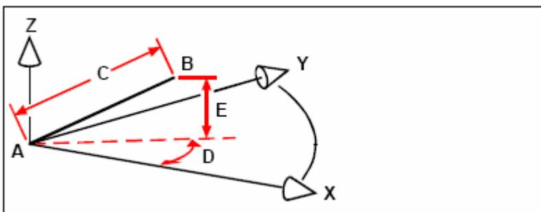
When you draw a line from a start point (**A**) to an endpoint (**B**) using cylindrical coordinates, you specify its length (**C**, in this case 7.4750), the angle in the xy plane (**D**, in this case 27 degrees), and the distance in the z direction (**E**, in this case 3 units).
