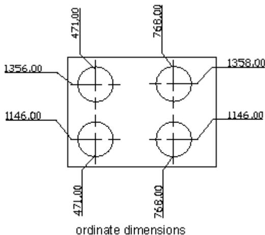
X ordinate dimensions show the distance of a feature from the datum along the X axis. And Y ordinate dimensions show the distance along the Y axis. The system determines whether the dimension is X or Y ordinate dimension depending on the point you specify. If the distance is greater for the Y value, the system creates an X ordinate dimension. Otherwise, the system creates a Y ordinate dimension.
