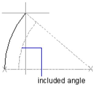
The included angle determines the endpoint of the arc. Use the Start, End, Angle method when you know both endpoints but cannot snap to a center point.
