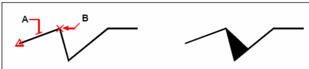
Select the polyline (**A**), move the current vertex marker to the first vertex of the segment you want to taper (**B**), and then specify the new starting and ending widths for that segment.
