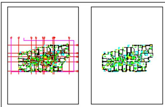
Once frozen, the layer in the viewport is invisible. With the layer thawing, its visibility can be restored. User can control the frozen status of layers by clicking Freeze in current viewport option in layer property manager.
