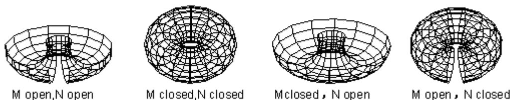
Various methods are used for creating mesh, both using keyboard way to specify mesh parameter or operating 3D command to draw planar mesh, The size of *M* and *N* of a mesh determines the number of lines drawn on each direction.
