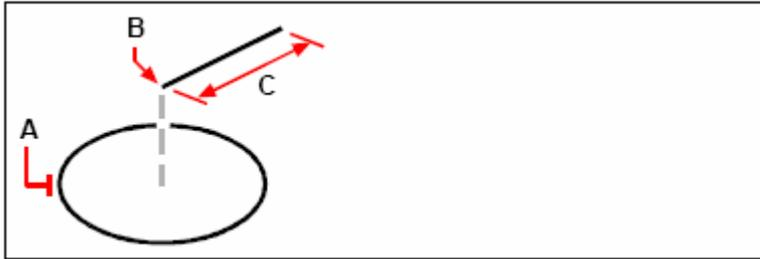
You can use point filters to draw a line by first selecting a point in the xy plane (**A**), specifying the z coordinate (**B**), and then specifying the length of the line (**C**).
