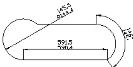
The vertical placement of tolerance values that is relative to the main dimension text can be specified. For example, you can align the tolerances with the top, middle, or bottom of the dimension text.
