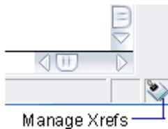
If the original drawing to which the xref links has been changed and needs to reload, an exclamation mark appears on the xref icon.
