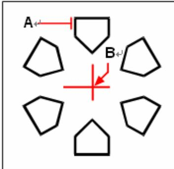
To create a polar array, select the object to copy (**A**), specify the center point of the array (**B**), and then specify the number of items to array, the angle the array is to fill, and whether to rotate the items.
