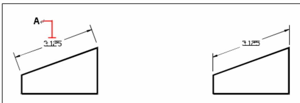
Select the dimension to be made oblique (A), and then type the obliquing angle.
