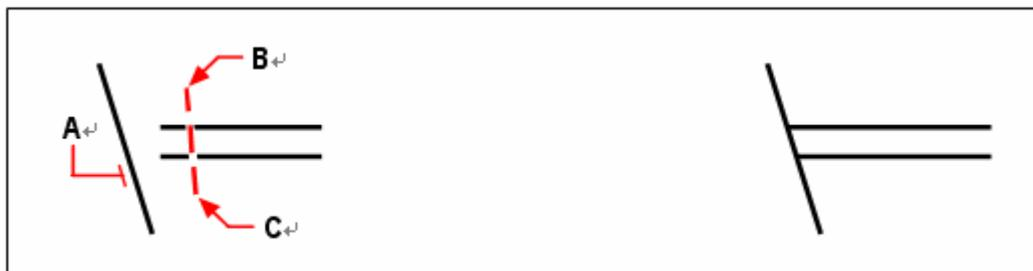
Select the boundary edge (**A**), and then specify the first point (**B**) and second point (**C**) of the fence.
