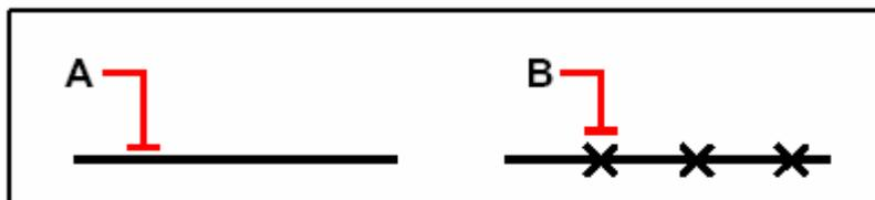
When you select the object by pointing, intervals are measured from the end closest to the point at which you select the object (A)
