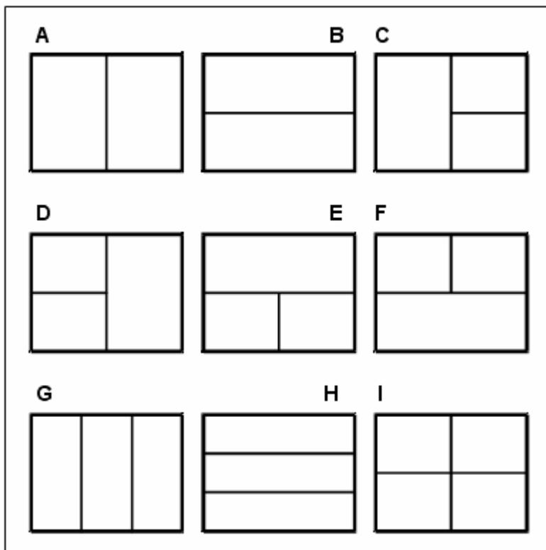
You can divide a drawing window into two windows arranged vertically (**A**) or horizontally (**B**); three windows arranged left (**C**), right (**D**), above (**E**), below (**F**), vertically (**G**), or horizontally (**H**); or four tiled windows (**I**).
