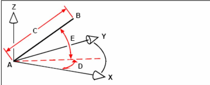
When you draw a line from a start point (**A**) to an endpoint (**B**) using spherical coordinates, you specify its length (**C**, in this case 10.2500 units), the angle in the xy plane (**D**, in this case 45 degrees), and the angle from the xy plane (**E**, in this case 35 degrees).
