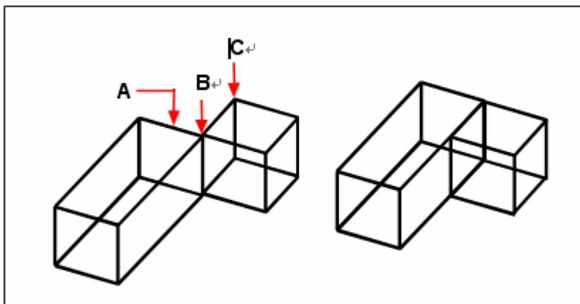
Specify the face(s) to move (A), the base point (B), and the end point (C). The resulting object with the face moved to the new position.
