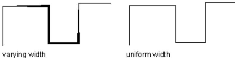
If you chose Width option, prompts in command line require you to enter starting width and ending width. While entering different value results in a varying width from the start point to its end. Both the start point and endpoint are located at the center of Wide polyline.
