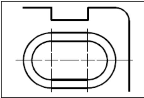
Snap and entity snap force the cursor to adhere to a specified increment or attach to key geometric points on existing entities. You can also constrain lines to vertical and horizontal axes.
