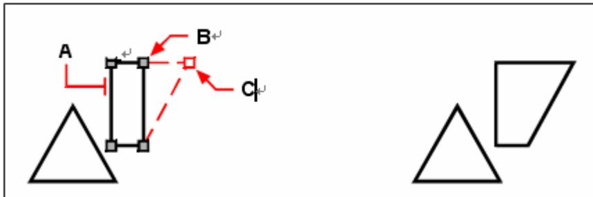
To stretch an object using grips, select the object (**A**), select a grip (**B**), and drag the grip to its new location (**C**).
