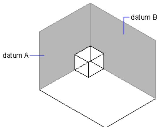
In the illustration above, the axis formed by the point where datums A and B intersect called the datum axis. The position of the pattern is calculated from that axis.
