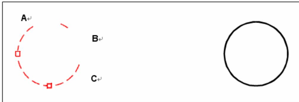
To scale using grips, select the object (**A**), click a grip (**B**), and scale the object by dragging the grip to its new location (**C**).
