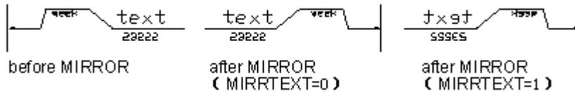
By default, the MIRRTEXT is on. It affects text objects created with TEXT, ATTDER, METEXT command as well as attribute definition and variable attribute. Text as well as constant attributes that are included in an insert block are mirrored together with the block while mirroring.
