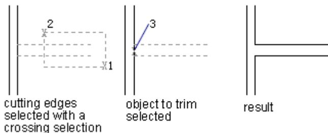
Using variable selection methods while trimming several objects can help you select edges or objects more easily.
