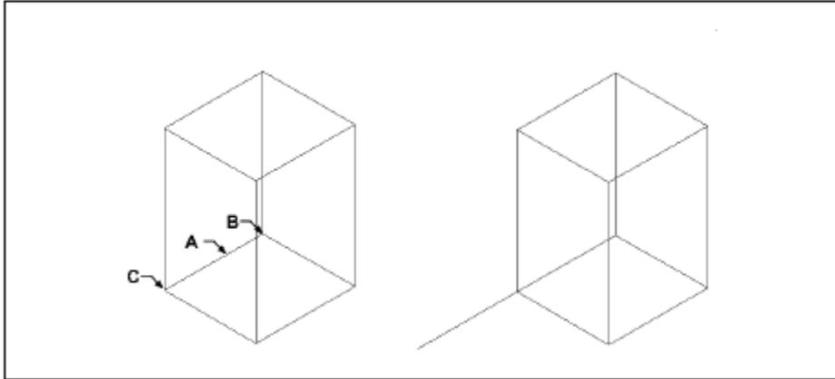
Specify the edge(s) to copy (**A**), the base point (**B**), and the end point(**C**).
