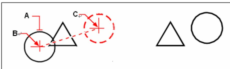
To move an object, select it (A), and then specify the base point (B) and the displacement point (C). Result
