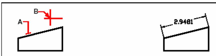
To insert an aligned dimension by selecting the entity, select the entity (**A**) to dimension, and then select the dimension line location (**B**).
