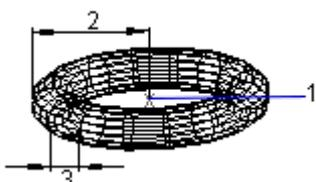
You can draw a torus with no center hole called self-intersecting torus because the radius of the tube is greater than the radius of the torus. To create a bipolar-depression solid, specify a positive tube radius greater than the radius of torus. 3D command creates a toroidal shape defined by surfaces only.
