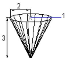
You can draw a 2D circle and then use EXTRUDE to taper the circle at an angle along the Z axis to create a solid cone.
