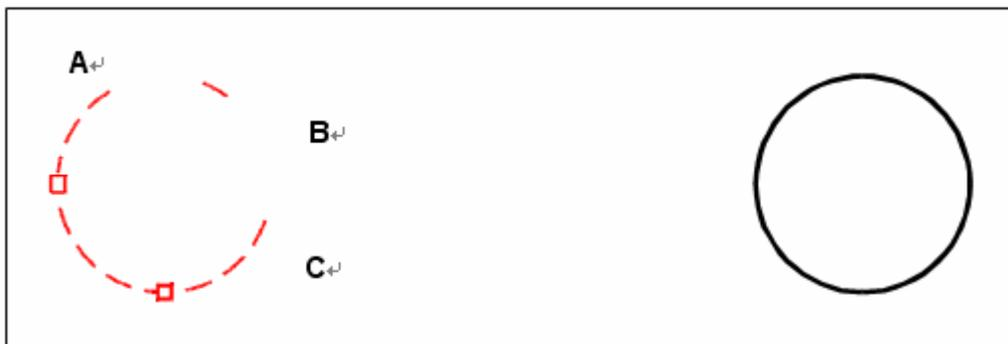
To scale using grips, select the object (**A**), click a grip (**B**), and scale the object by dragging the grip to its new location (**C**). Result.
