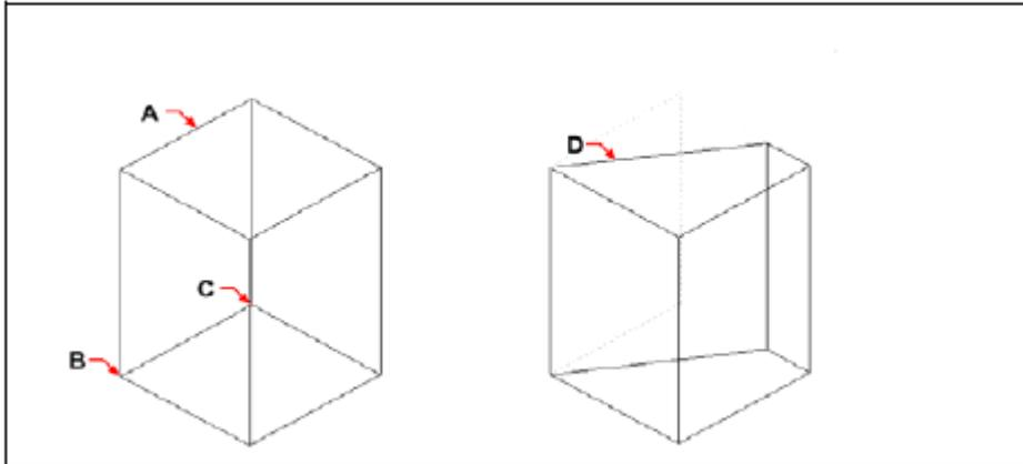
Specify the face(s) to taper (**A**), a base point(**B**), a second point position(**D**), along the taper axis(**C**), and a taper angle.
