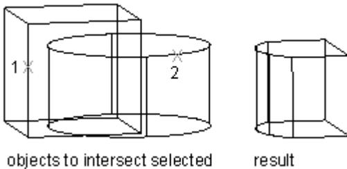
Unlike INTERSECT command, INTERFERE compares the objects among two selected sets and creates composite entity with common volume of two or more solids without removing the original objects.
