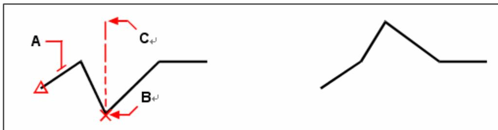
Select the polyline (A), move the current vertex marker to the vertex you want to move (B), and then specify the new vertex location (C).
