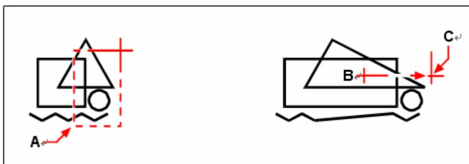
To stretch objects, select them using a crossing window (A) or crossing polygon, and then specify the base point (B) and displacement point (C).
