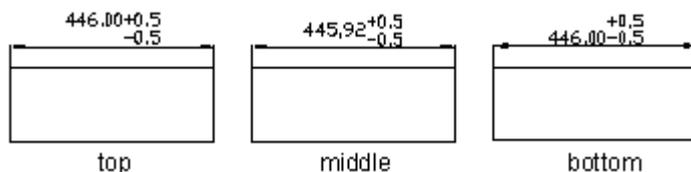
You can also control how to suppress zero for tolerance values, as you can with the primary and alternate units. The effect of suppressing zero in lateral tolerance is the same as suppressing zero in the primary and alternate units.
