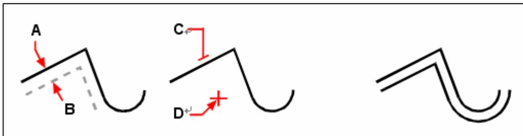
To make a parallel copy, specify the distance between copies by entering a distance or selecting two points (**A** and **B**), select the object to copy (**C**), and specify on which side to place the copy (**D**). Result.
