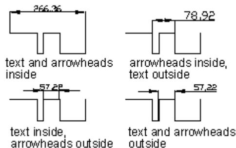
If there is no space for text between the extension lines, the system creates a leader automatically to place text. You can set the relationship between them on the Text tab of the Modify Dimension Style dialog box.
