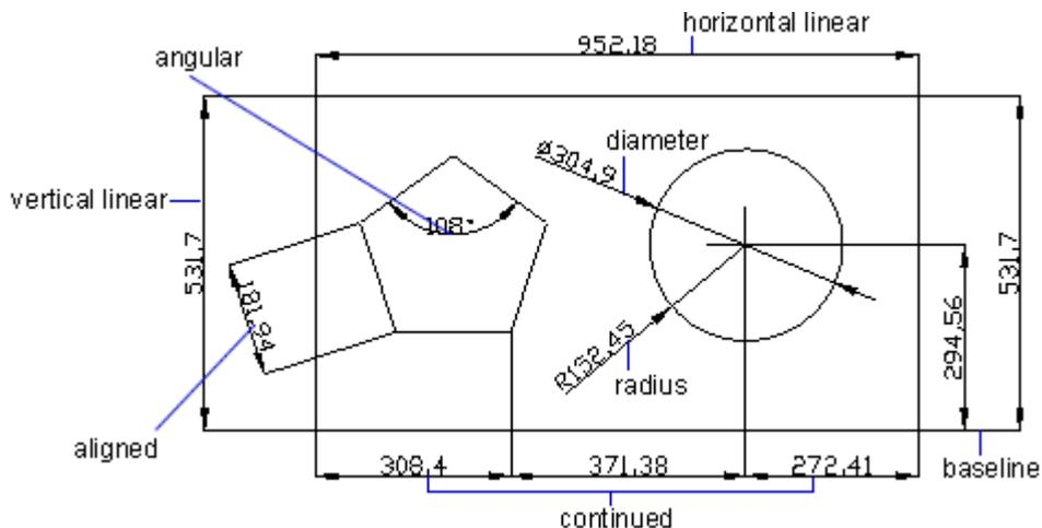
When you create a dimension, the program draws it on the current layer, using the current dimension style. Each dimension has an associated dimension style, which controls the appearance of the dimension, such as the types of arrowheads, text style, and colors of various components. You can modify existing dimension styles by changing any of the dimension variable settings, and the new dimension style is visible soon after you confirm the modification.
