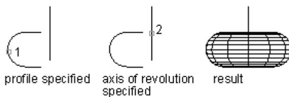
You can create a surface of revolution, which is a three dimensional polygon mesh that approximates the surface generated by rotating a two dimensional profile around an axis. You select the two objects that define the profile and the axis. You also specify the starting angle and the number of degrees to revolve the profile.
