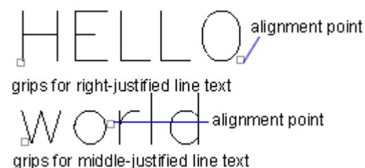
Different grips generate different effect even though with the same command.
