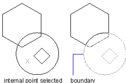
With the Boundary command, you can designate a specific area of a drawing for operations such as hatching and dimensioning. You create a boundary polyline by selecting an area inside a closed loop. The area you select can be bounded by a single closed object or by multiple objects that intersect.
