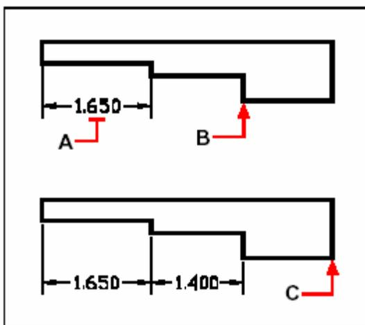
To add a continued dimension to an existing linear dimension, select the existing dimension (A), select the next extension line origin (B), and select another extension line origin (C).
