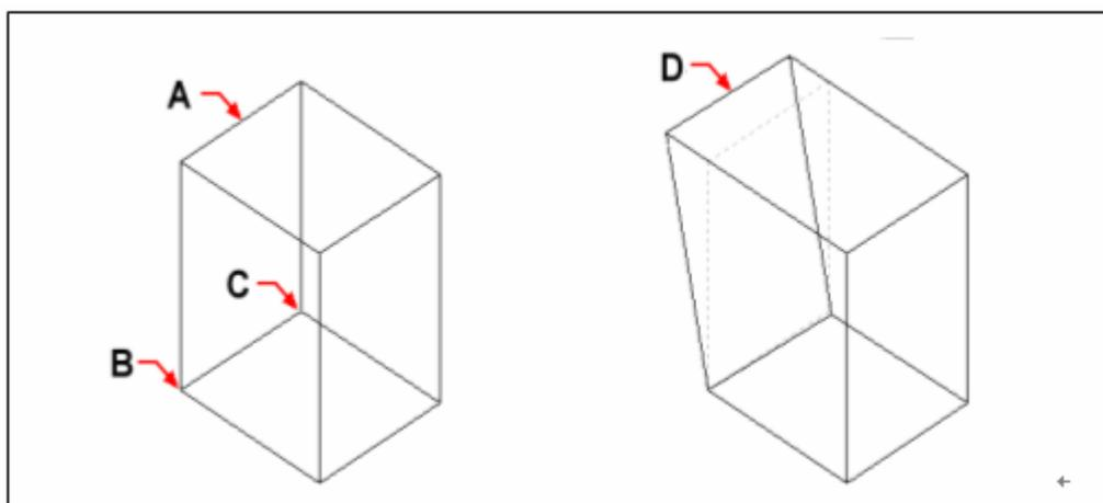
Specify the face(s) to rotate (**A**), the base point (**B**), a second point on the rotation axis (**C**), and a rotation angle.
