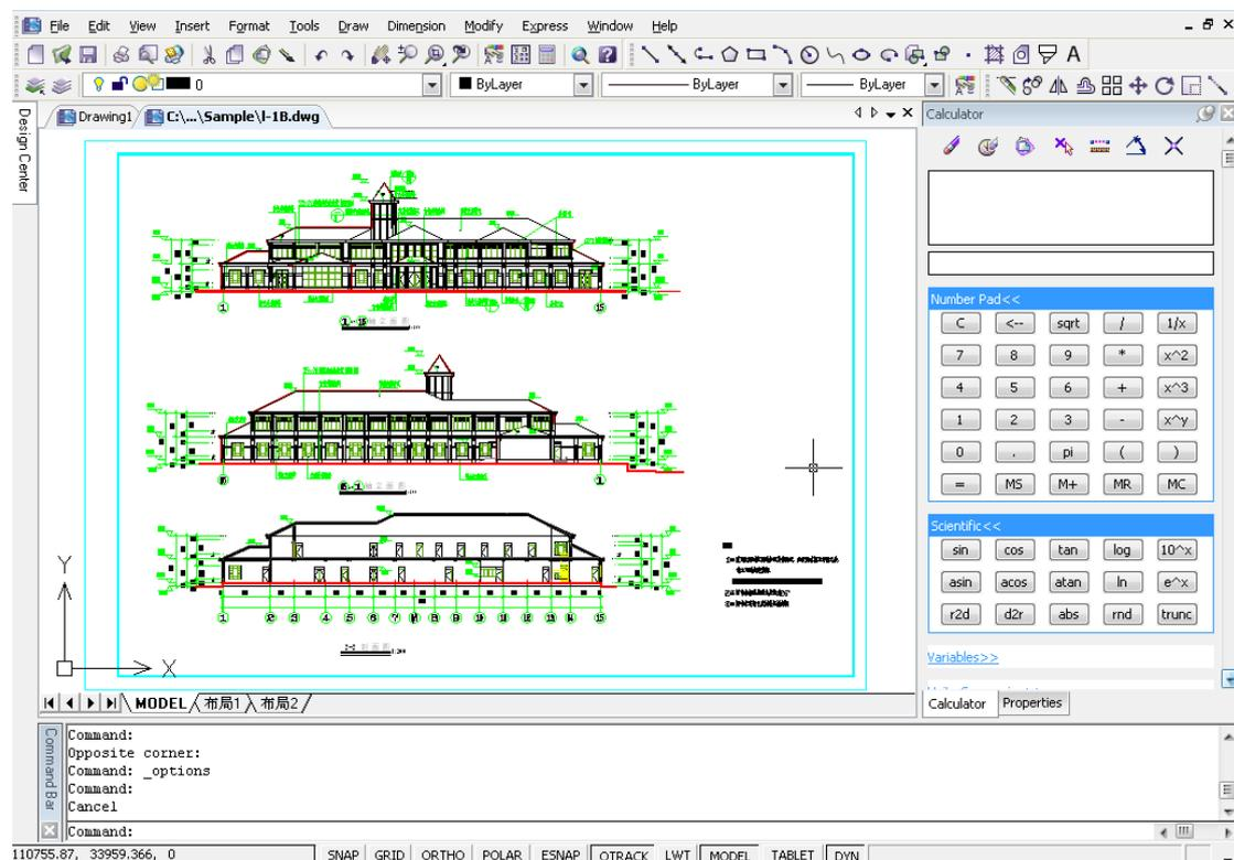
You create the basic drawing in model space on the Model tab.
